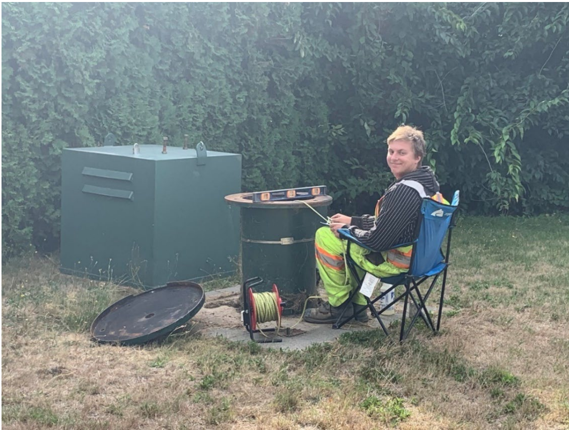
IMAGE | WATER LEVELS ARE TAKEN BY CWD STAFF DURING WELL TESTING.
